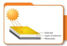
The selenium PV cell produced a small amount of electricity when placed in direct sunlight.
