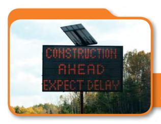
This road sign is powered with a PV system.
