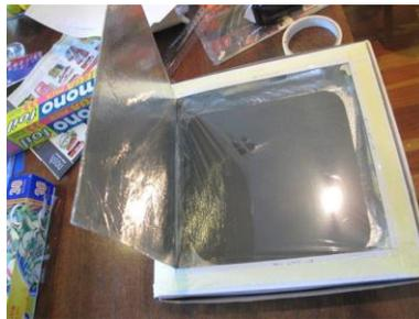
15. To adjust the angle of the solar reflector so that it reflects as much light as possible into the oven you can use a piece of masking tape attached to the back of the box. Alternatively use a ruler and string, blu-tak etc.
