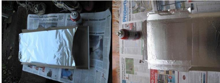
3. Put some glue (spray glue is useful) on the bottom of the box at one end and then smooth the foil carefully onto the cardboard.
