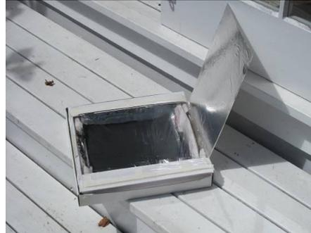
3. Open the box, place the food to be heated in the centre (a small square of cooking paper underneath keeps the oven clean), and close the box.
